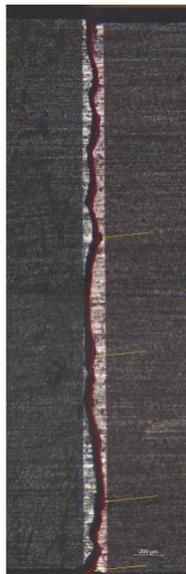
Figure 5: location of the failure in the braze (SEM F4P sample CEA 1 100 $\mu\text{m}$ )
