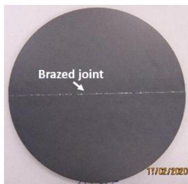
Figure 2: Brazed sample before machining ( $\phi$  100 mm, h 3,9 mm).
