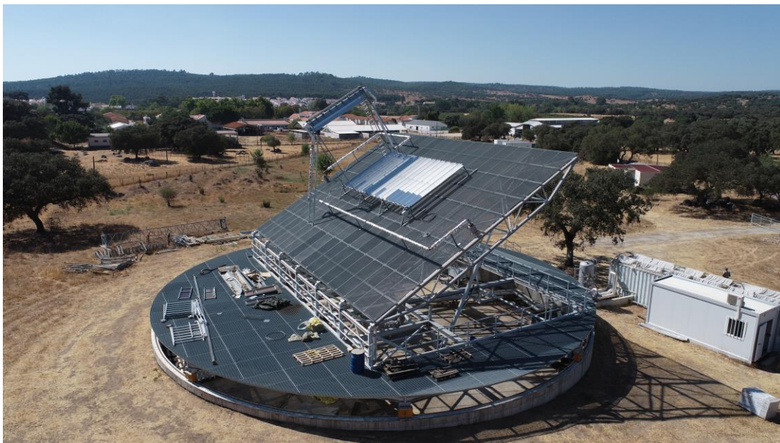
Figure 7: The experimental test of the ALFR collector using the PECS platform.
