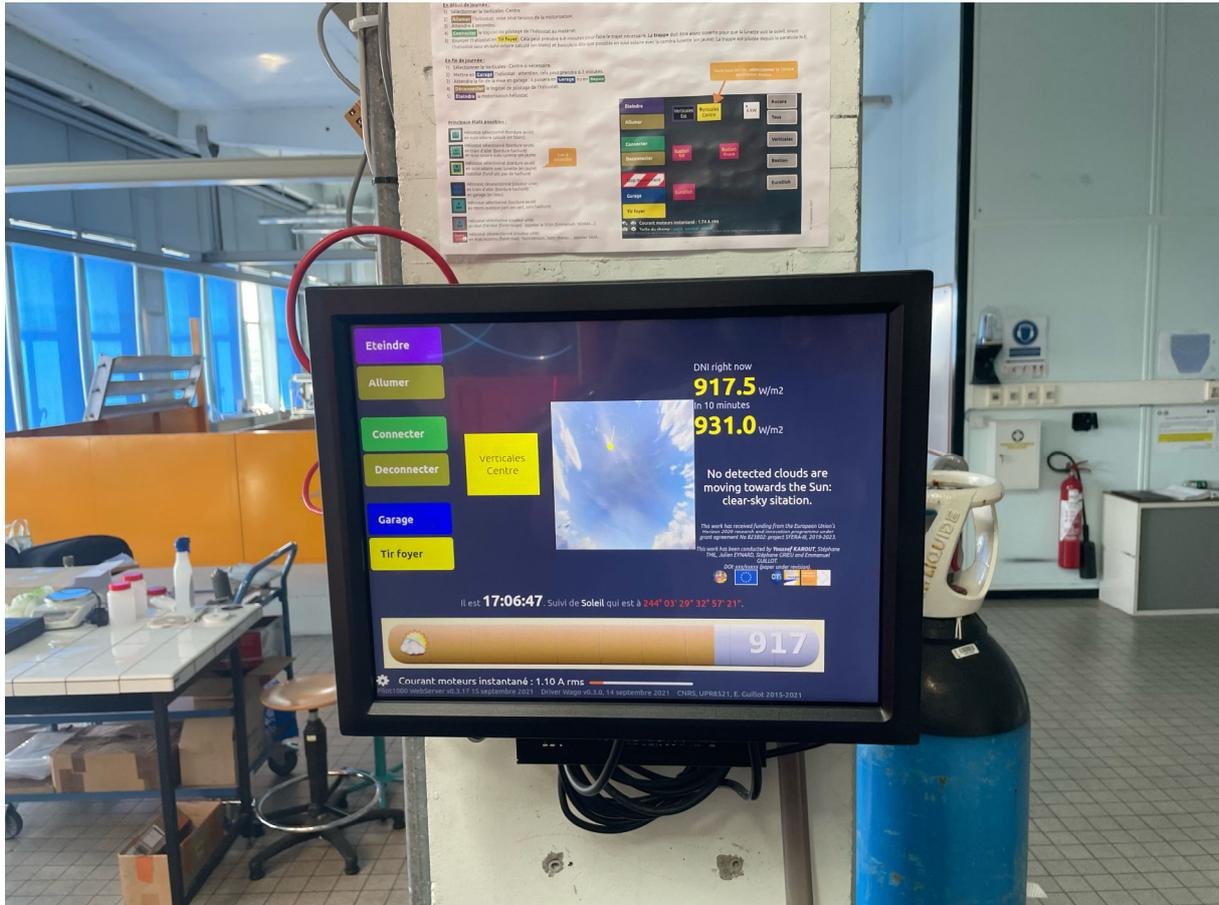
Figure 13. **The GUI providing DNI forecasts to RI users in Odeillo, France.**
