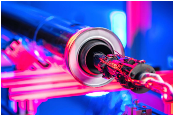
Parabolic Trough Receiver being prepared with a heater in a heat loss test rig
