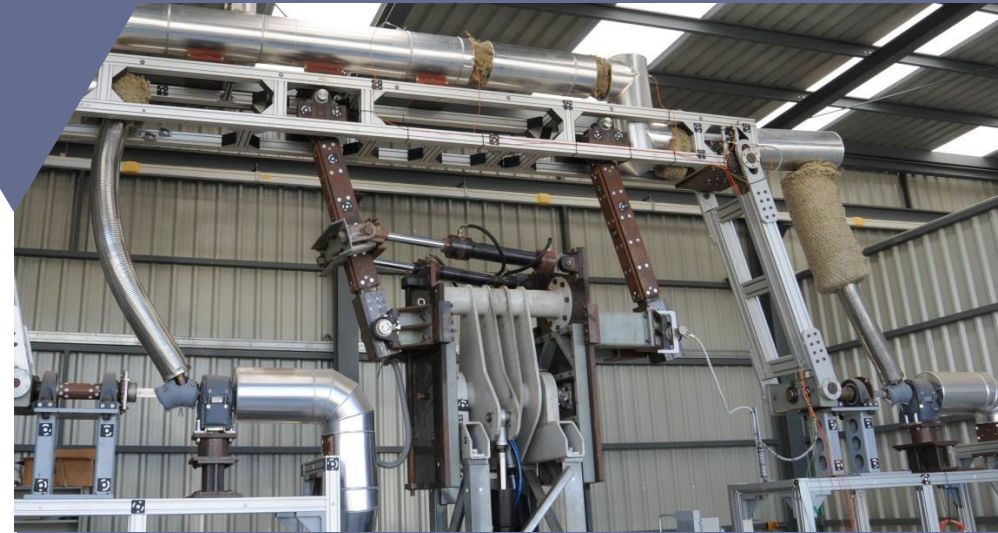
DLR calibration adapter for load cells (dynamometer) on REPA test rig
