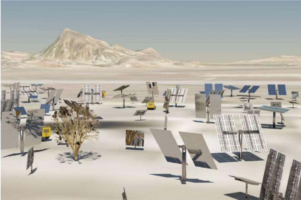
Fig.1. Example image from our simulation environment. The random compilation of our scenes helps to overcome the reality gap when training deep learning models.
