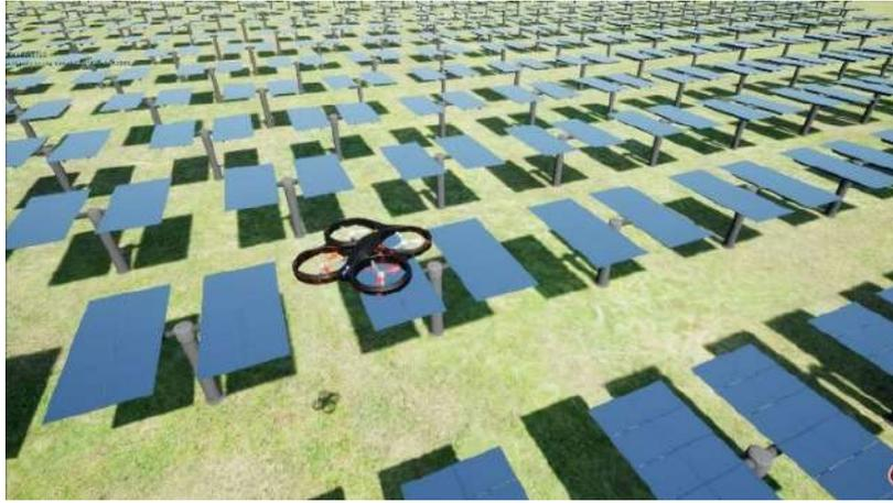
Fig.1. The simulated drone is controlled inside a virtual environment. The simulation allows for the modeling of a heliostat field and real-time sampling of both, camera position and image data.
