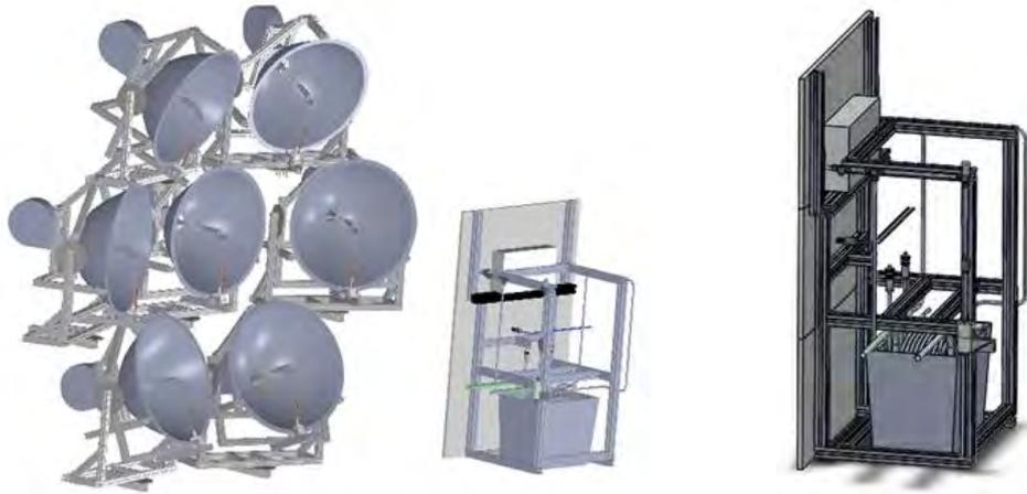
Fig.1. Experimental facility developed for gas phase receiver testing. (Left) KIRAN-42 High Flux Solar Simulator; and (right) Calorimetric testbed for receiver evaluation.
