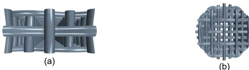
Fig. 1. Studied arrangements for pressure drop: (a) Rectangular and (b) Circular.
