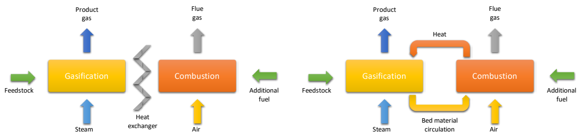
Figure 9. Allothermal process only with heat exchange.
