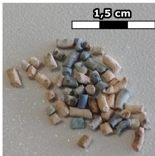
Figure 13. **Photograph of part of the particles recovered after hydrogen production experiments**
