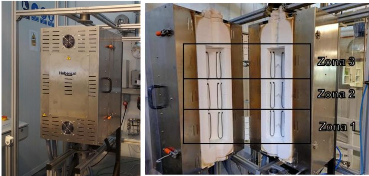
Figure 7. **Vertical tube furnace ST-6V3Z**
