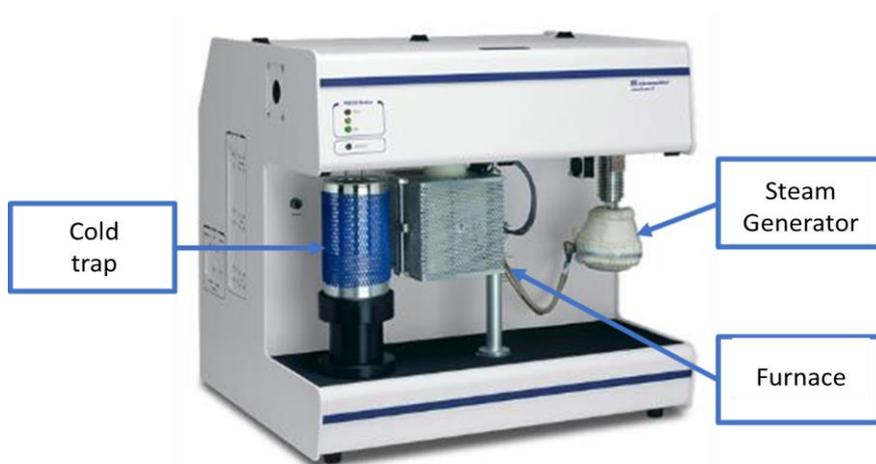
Figure 1. **Chemisorption equipment AutoChem II 2920 from Micrometrics.**
