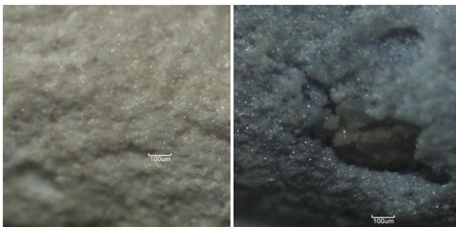
Figure 14. **Optical micrographs of ceria particles used for hydrogen production: (a) pink particles (b) blue particles**
