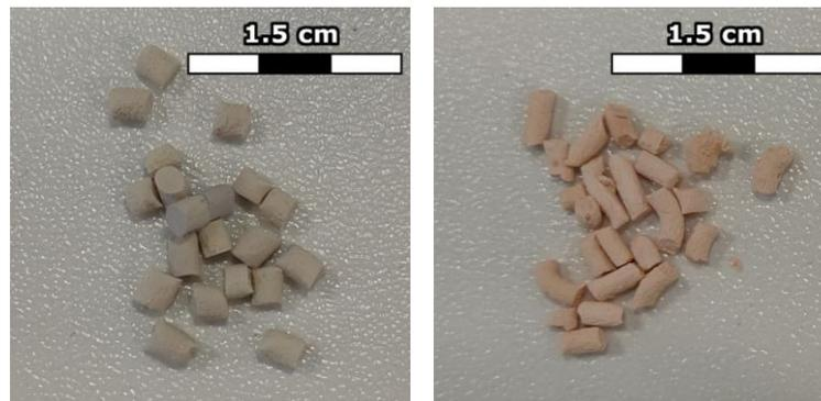
Figure 10. **Photos of (left) overnight-dried and (right) sintered fresh ceria pellets**
