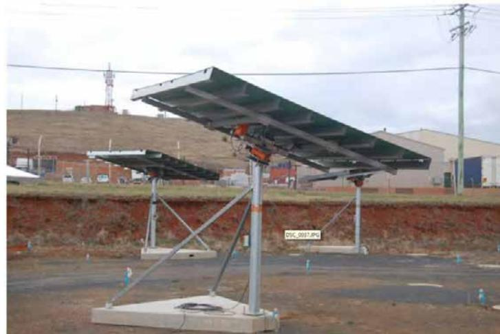
Heliosystems's 9m<sup>2</sup> "Passive Adjustment Toroidal Heliostat" (PATH),
