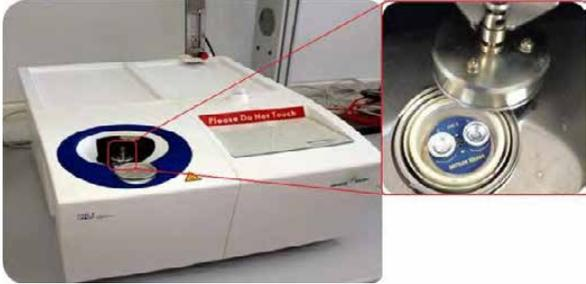
Applying a controlled temperature ramp on a Al pan 100 ul, filled with salt allowing the salt to melt and then to solidify it is possible to detect “onsets” of solidification and melting (T<sub>liq</sub> and T<sub>sol</sub>)
