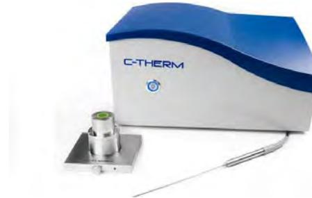
A known current is applied to the sensor's heating element providing a small amount of heat. The heat provided results in a rise in temperature at the interface between the sensor and the sample.
