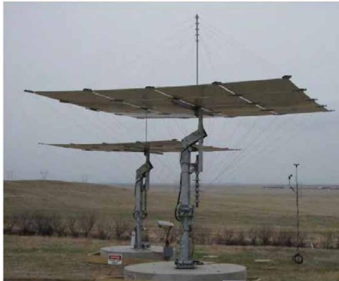
Solaflect's 16 m<sup>2</sup> 'suspension heliostat'. 16 x 1 m<sup>2</sup> glass facets held in position by cables tensioned from a compression element perpendicular and central to the mirror panels
