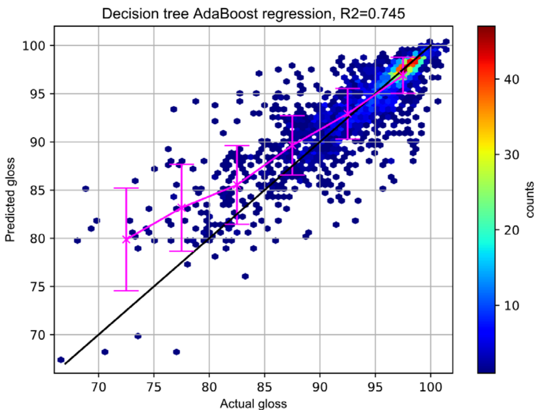
Fig. 1. Validation data of gloss prediction from regression decision tree with adaptive boosting
