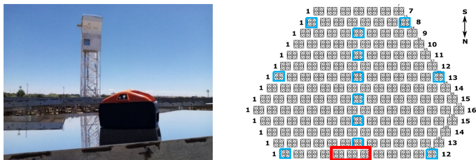
Fig. 1: a) Condor reflectometer with the VHCST on background; b) IMDEA's solar field layout with blue squares marking heliostats measured with tilt of 3° and red rectangle marking heliostats tilted 0°, 15° and 30°.
