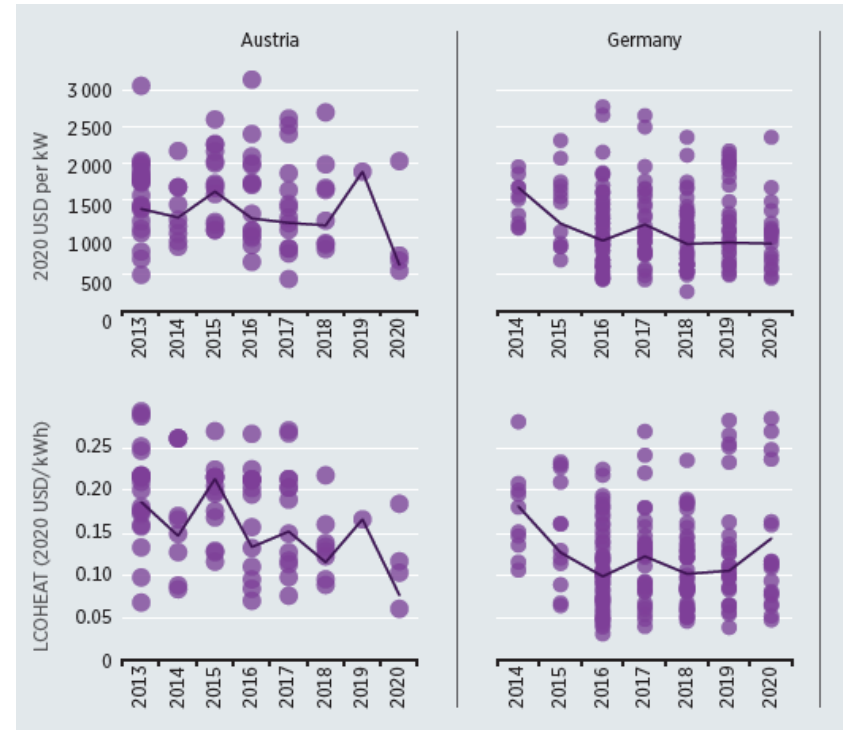
Total installed costs and LCOHEAT for commercial and industrial-scale solar thermal plants in Austria and Germany, 2010-2020
