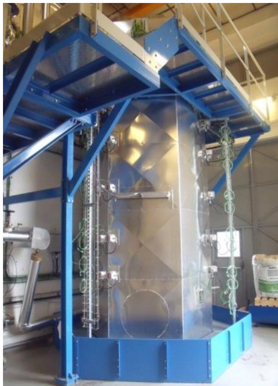
Figure 13. LHASSA: A PCM storage prototype + HP Steam loop.
