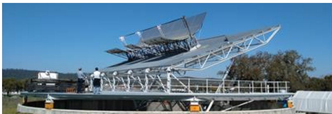
Figure 14. Two-axis solar platform (PECS) for the testing of solar concentrators modules up to 400°C with oil loop.
