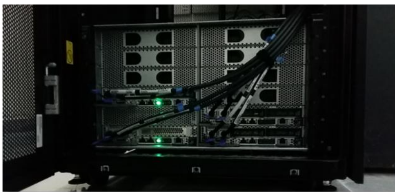
Figure 27. HPC Cluster with 96 computation cores, 768 GB of RAM, 32 TB for storage and an Infiniband (56 Gb/s) communication infrastructure and nodes for MPI computation.
