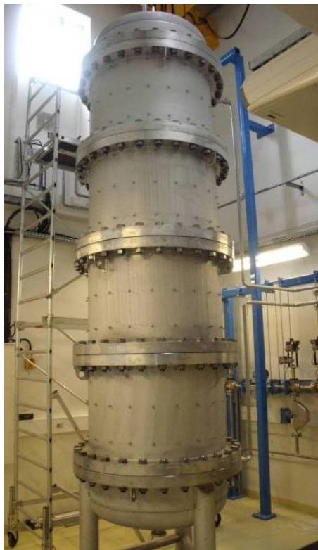
Figure 12. STONE: A dual media thermocline storage prototype + Oil loop.
