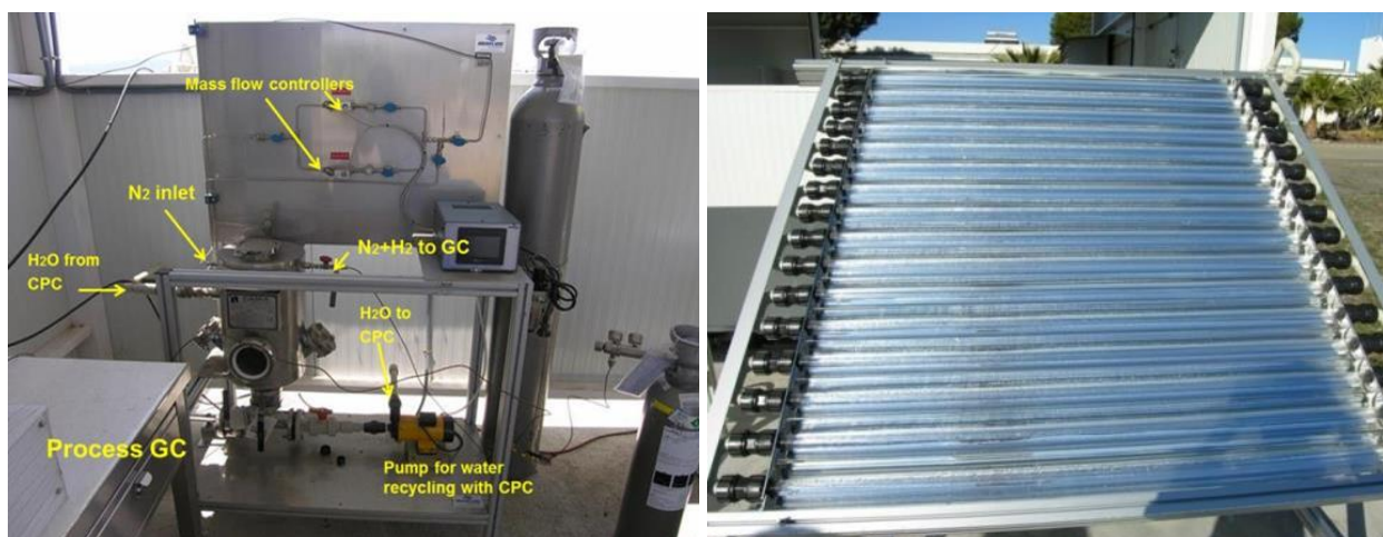
Figure 6. Solar pilot plant for photocatalytic generation of hydrogen (left) and CPC photo-reactor (right).
