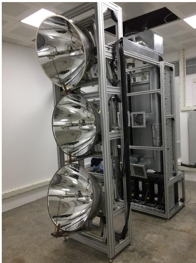
Figure 28. GunSolSim: ODAK High Flux Solar Simulator
