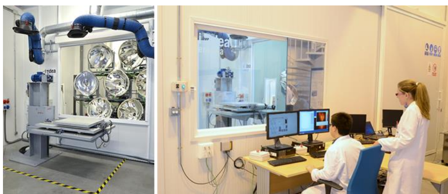
Figure 17. 42kWe High Flux Solar Simulator (KIRAN42).
