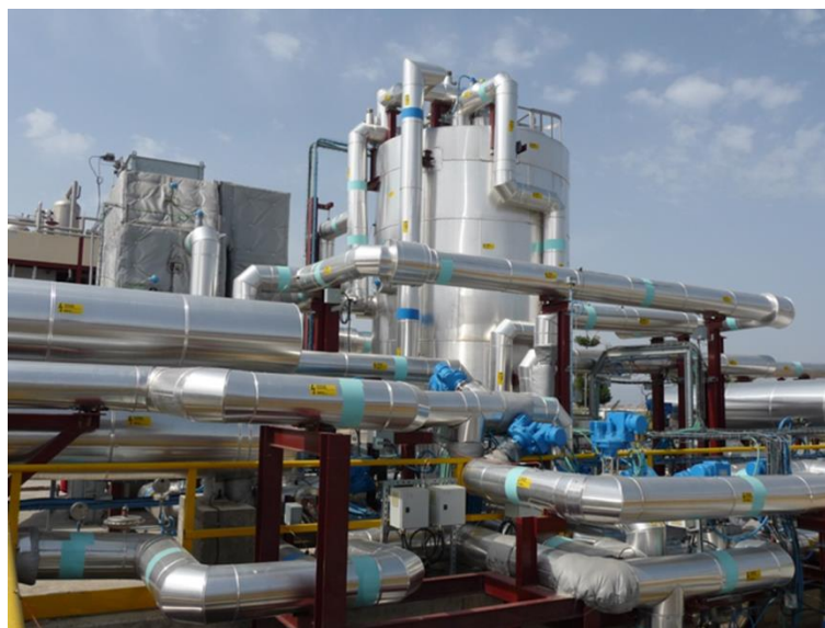
Figure 3. MOlten SALT test loop for Thermal Energy Systems (MOSA).
