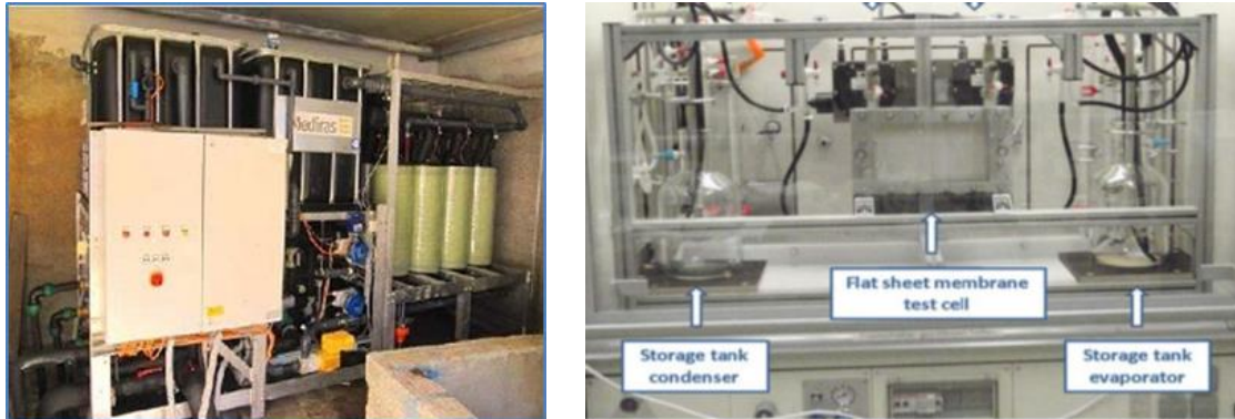
Figure 23. Membrane distillation field operation testing plant (Left). Flat membrane test facility for aggressive media (Right).
