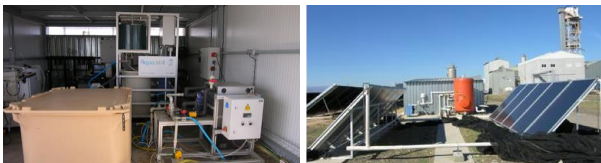
Figure 8. Internal (left) and external (right) views of the Membrane Distillation experimental test bed within the PSA low-temperature solar thermal desalination facility.
