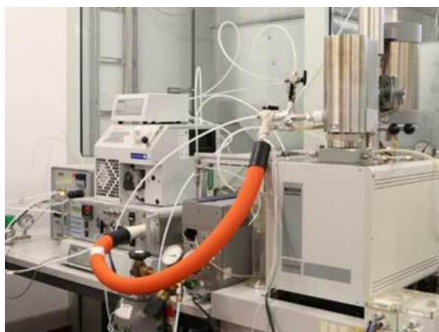
Figure 16. The Netsch TGA from the CHEM installation, with a gas chromatography system monitoring the outlet gas.
