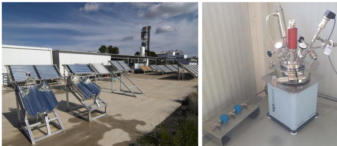
Figure 4. CPC in the Solar Water (SolWat) pilot plant (left) and Wet Air Oxidation (WetOx) pilot plant (right).
