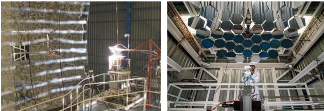
Figure 1. Interior view of the PSA SF60 Solar Furnace in operation (left) and Interior view of the PSA SF5 Solar Furnace (right).
