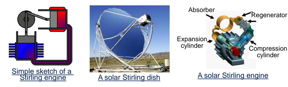
The two main benefits of Stirling engines are their high thermal efficiency (>30%) and the absence of pollutant combustion gases
