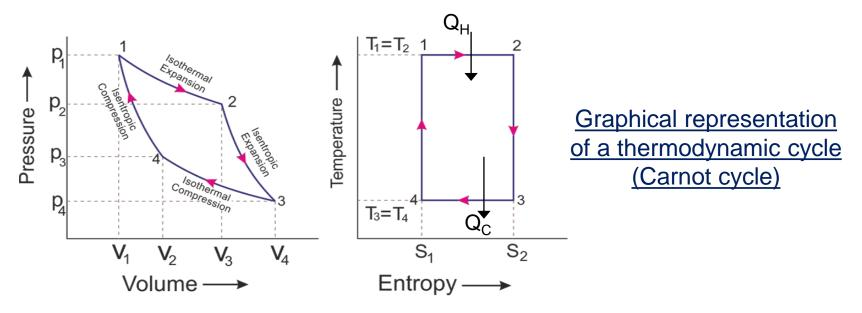
During a thermodynamic cycle the system can exchange heat and/or mechanical energy (work) with its surrounding
