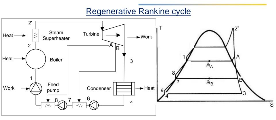
The cycle efficiency is increased by raising the mean cycle input temperature. The working fluid in the cycle is heated by steam extractions from the turbine. Although the more steam extractions the higher the efficiency, **there are practical limitations** due to the cost of the regenerators.
