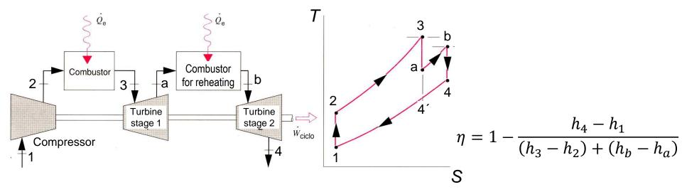
➤ Although the net mechanical work is higher the thermal energy consumption is higher too → the efficiency is not necessarily higher than that of a basic Brayton cycle. The efficiency will be higher than the basic cycle only if T<sub>b</sub>-T<sub>a</sub> > T<sub>4</sub>-T<sub>4</sub>.
