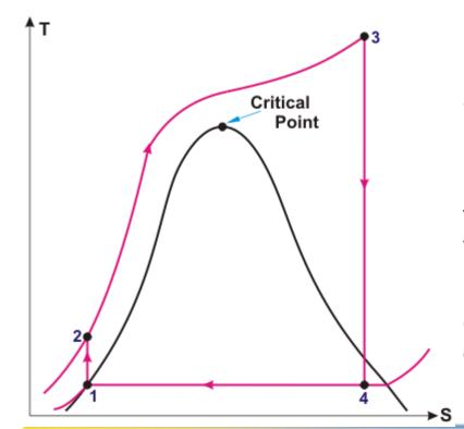
> The main benefit of a SBC is a higher efficiency that a superheated Rankine cycle  $(43\% \rightarrow 46\%)$
