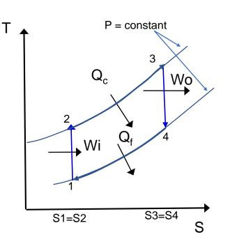
Compression thermal ratio  $\lambda = \left(\frac{P_2}{P_1}\right)^{\frac{\gamma-1}{\gamma}}$
