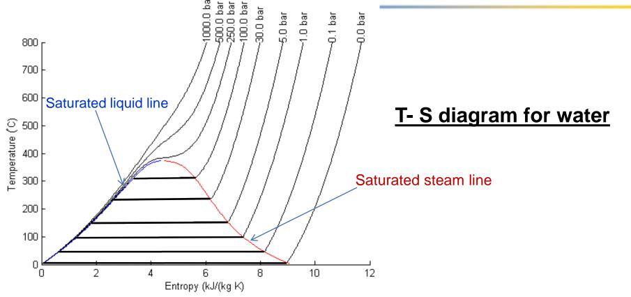
When liquid water is heated at constant pressure, the water increases its temperature until the saturation temperature is reached. At that moment, water starts boiling and passing from liquid to steam phase without increasing its temperature (<u>liquid+steam</u>). When all water is in gas phase it increases its temperature (<u>superheated steam</u>)
