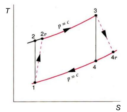
$$\mu_{C} = \frac{W_{IC}}{W_{RC}} = \frac{h_{2} - h_{1}}{h_{2R} - h_{1}}$$
