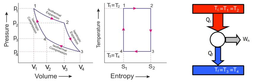
Since the four processes are reversible, this cycle is the cycle with the maximum possible efficiency for a thermodynamic cycle connected to the same heat source and heat sink:  $\eta_{\text{Carnot}} = \eta_{\text{max.}} = 1 - \frac{T_f}{T_c} < 1$
