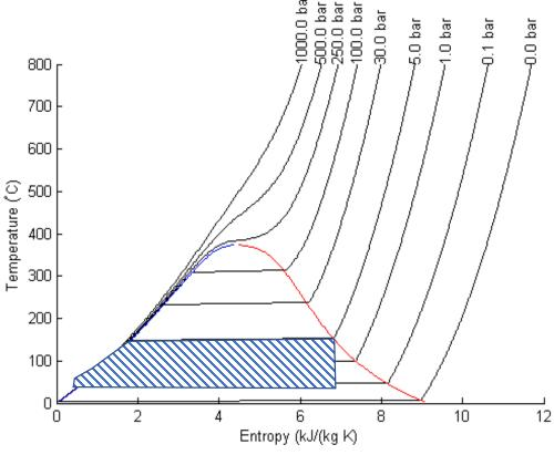
When the temperature of the heat source available is low (T<150°C) the use of water for a Rankine cycle is not good because of two main problems:
