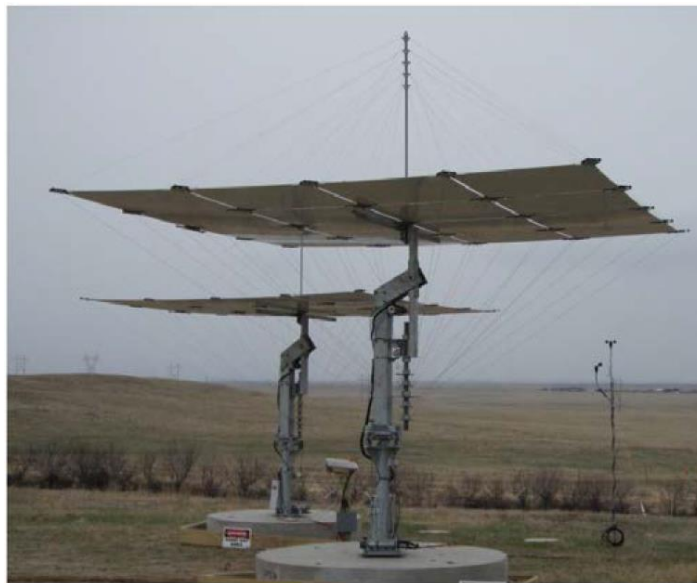
Solaflect's 16 m 2 'suspension heliostat'. 16 x 1 m 2 glass facets held in position by cables tensioned from a compression element perpendicular and central to the mirror panels
