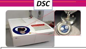
Applying a controlled temperature ramp on a Al pan 100 ul, filled with salt allowing the salt to melt and then to solidify it is possible to detect **"onsets**" of solidification and melting (Tliq and Tsol)
