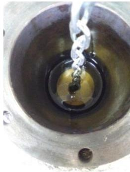
The method is based on the measurement of the buoyance force on a stainless steel cylinder, which is immersed into the ternary melt and is connected with a dynamometer.
