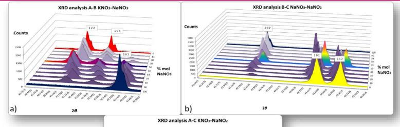
A modification of the distance between the crystallographic planes is related, considering that  $\lambda$  is constant, to a change in the 20 values.
