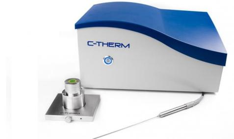
A known current is applied to the sensor's heating element providing a small amount of heat. The heat provided results in a rise in temperature at the interface between the sensor and the sample.
