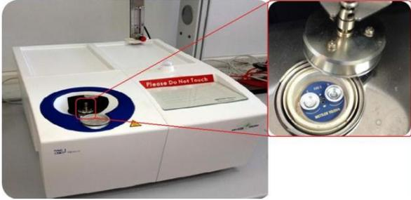
Applying a controlled temperature ramp on a Al pan 100 ul, filled with salt allowing the salt to melt and then to solidify it is possible to detect "onsets" of solidification and melting ( $T_{liq}$  and  $T_{sol}$ )
