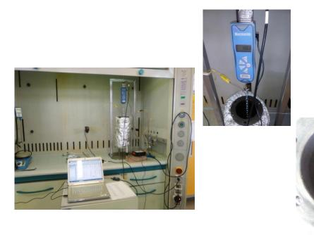
The method is based on the measurement of the buoyance force on a stainless steel cylinder, which is immersed into the ternary melt and is connected with a dynamometer.  ✓ Heat conductivity : instrument based on the "hot wire" method (up to 80°C)
