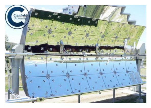
*Experiment*: Photogrammetry targets were attached to a single parabolic trough module, and photographs were taken by multiple operators and cameras from a range of locations. The trough was moved to different tracking positions and measurements were made at each position.
