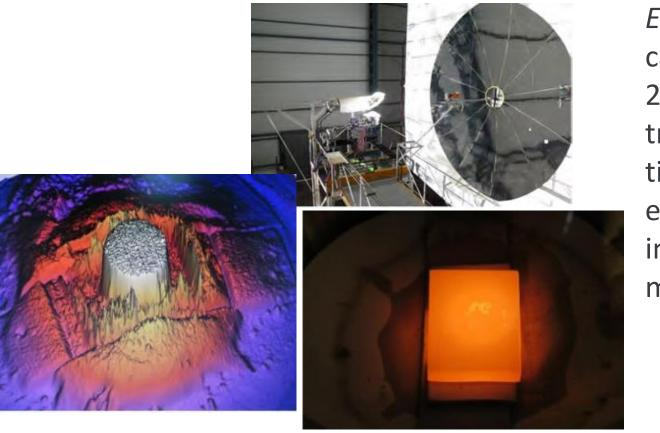
*Experiment*: The three solar test campaigns carried out in the SF40 solar furnace between 2014 and 2016 were successful for all applied treatment parameters (type of powder, dwell time and atmosphere). Also, special experiments were carried out in order to investigate the influence of post-elaboration remelting (double solar exposure)
